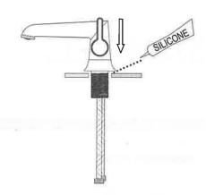
Reinstall rubber washer and metal washer from below. Hand tighten lock nut from below while aligning fixture.
