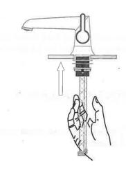
4 Secure fixture below by using either an adjustable wrench, basin wrench, or deep socket to the lock nut. Wipe away excess silicone with a wet finger or damp cloth. Connect flexible hoses to their respective water supplies.
