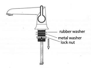
Apply a ring of silicone caulking around hole designated for spout. DO NOT USE PLUMBERS' PUTTY WHICH CAN DAMAGE FINISH. Insert faucet assembly through hole in sink or counter top, being sure to center faucet in hole.
