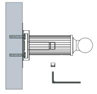
Using the allen key provided, loosen the set screws from the bar posts.
