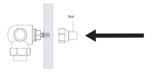
Insert the broach into the valve. Then fit the all thread over the broach and hand tighten it into the nut until it bottoms out.
