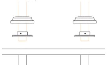
2. Mark the position of screw hole flange and remove both legs. Drill the pilot holes out for the screws at 5/16"
