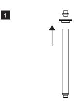
Step 1: Remove the nut from the top of the ceiling arm and slide the flange onto arm. Wrap Teflon tape around the threads and thread the nut back onto the arm.
