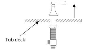
3 -Slip valve body up from below tub deck.
