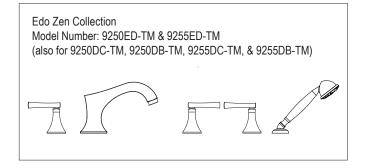
Flush both supply lines before installation, then shut off both supply lines. Minimum hole size for the spout and handle trim is 1-1/4" and maximum of 1-1/2"
