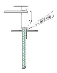
Reinstall rubber gaket and metal washer from below. Hand tighten fastening nut from below while aligning fixture.
