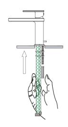
Secure fixture from below by using either an adjustable wrench, basin wrench, or deep socket to the lock nut. Wipe away excess silicone with a wet finger or damp cloth. Connect flexible hoses to their respedic water supplies.
