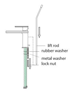
Apply a ring of silicone caulking around hole designated for spout. DO NOT USE PLUMBERS' PUTTY WHICH CAN DAMAGE FINISH. Insert faucet assembly through hole in sink or counter top, being sure to center faucet in hole.
