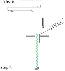
Secure fixture from below by using either an adjustable wrench, basin wrench or deep socket to the lock nut.
