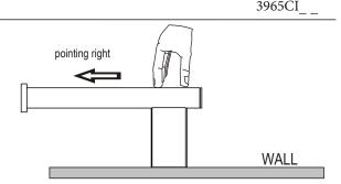
2- Using the Allen key provided, remove the mounting screw bracket from the holder post.
