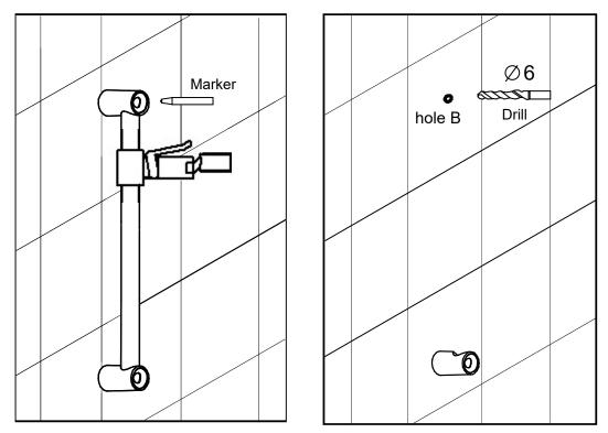
Step **7**: Inject the silicon into hole B and insert a toggle into it. Insert back the slide bar assembly all the way into the bottom post. Secure the top post to the wall using the screw(ST4X30).
