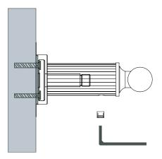
Using the allen key provided, loosen the set screws.
