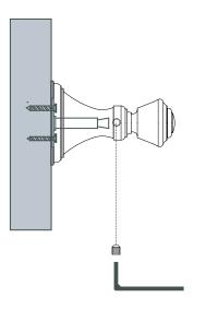
Using the provided Allen key, loosen the Accessory Post's Set Screw.
