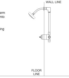
Step 1. Once shower arm is threaded into the wall , add Teflon tape to the threads.
