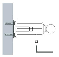
Using the allen key provided, loosen the bar posts' set screws.
