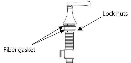
**2** - Remove the top lock nut and the fiber gasket from the valve body.
