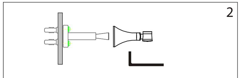
2. Set escutcheon over mounting bracket. Tighten setscrew with supplied allen key to secure.
