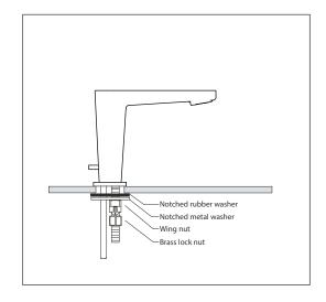
Align spout and secure to the sink or counter surface by tightening the 2 screws on the wing nut with a Phillips head screwdriver.
