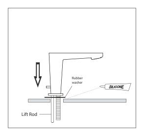
B Slip the spout mounting hardware back onto the spout. First the notched rubber washer, then the notched metal washer, (making sure the notch faces towards the back) wing nut, and brass lock nut. Insert lift rod and make sure it operates smoothly.
