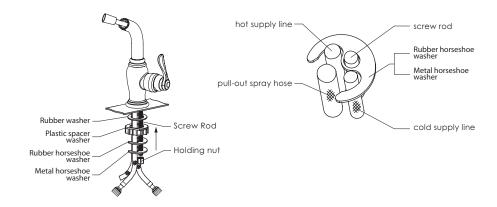
Insert and arrange the plastic hose guide in such a way that both spray hose and screw rod fit into the guide. Screw in the small holding nut to fix its position.
